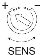
Adjust the Reach control to set the radius of operation of the microwave detection zone. An ideal ceiling mount height is 2.5m, turn the Reach control fully anti-clockwise to select the minimum reach (approx.1metre), and fully clockwise to select maximum reach (approx. 10metres).
