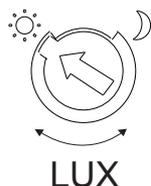
The chosen light threshold can be set from approx. 10-2000lux. Turn it fully anti-clockwise to select dusk operation at about 10 lux. Turn it fully clockwise to select daylight operation at about 2000lux. Turn the control fully clockwise when adjusting the motion detector sensitivity.
