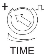
The light can be set to stay ON for any period of time between approx. 6sec (turned fully anticlockwise) and a maximum of 12min (turned fully clockwise). Any movement detected before this time has elapsed will re-start the timer. It is recommended to select the shortest time when adjusting the detection sensitivity.
